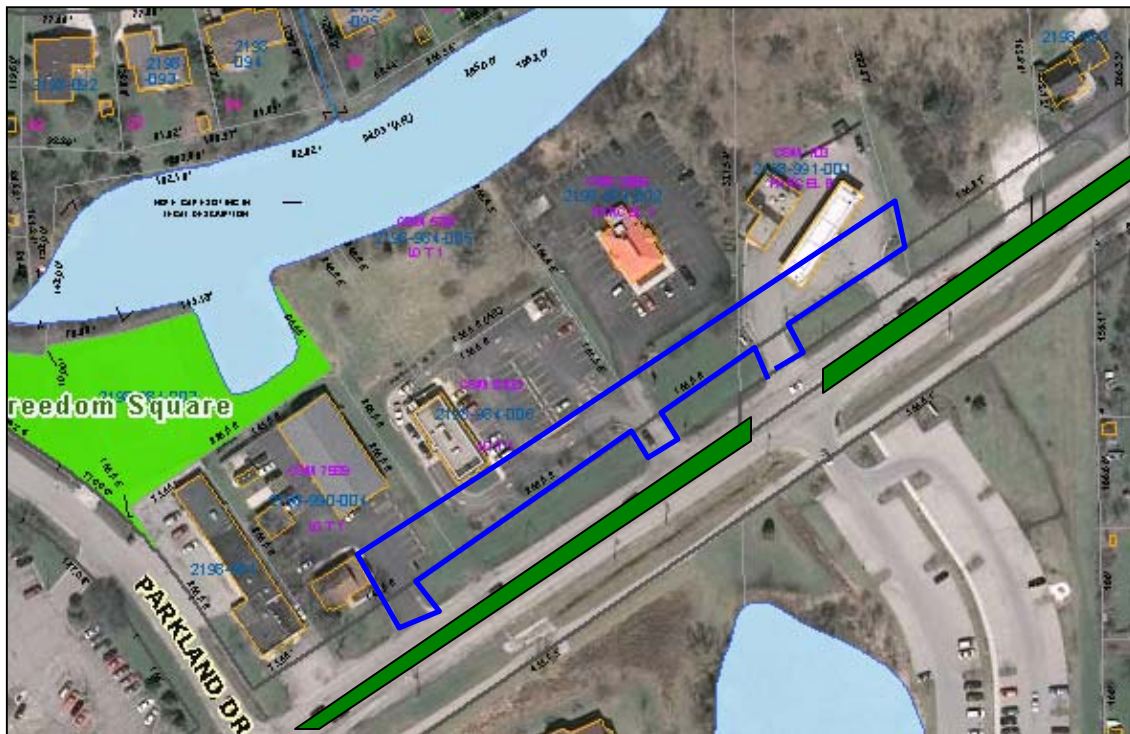
Fig. B: Since the new Janesville Road will have limited access (due to boulevard sections), linking cross access easements with new parking lot sections will benefit all businesses.
